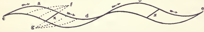
FIG. 13.—Wave track made by the wing in progressive flight. a, b , Crests of the wave; c, d, e , up strokes; x, x , down strokes; f , point corresponding to the anterior margin of the wing, and forming a centre for the downward rotation of the wing ( a, g ); g , point corresponding to the posterior margin of the wing, and forming a centre for the upward rotation of the wing ( d, f ).
